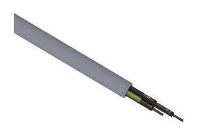
Southwire flexible control cable, unshielded, 4 conductors (includes ground), 20 AWG, bare copper, PVC/Nylon conductor insulation material, black with white numbers and green/yellow ground, TPE jacket, gray, cut to length.
