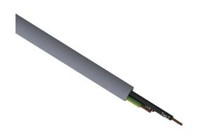
Southwire flexible control cable, unshielded, 3 conductors (includes ground), 20 AWG, bare copper, PVC/Nylon conductor insulation material, black with white numbers and green/yellow ground, TPE jacket, gray, cut to length.
