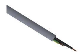
Southwire flexible control cable, unshielded, 3 conductors (includes ground), 20 AWG, bare copper, PVC/Nylon conductor insulation material, black with white numbers and green/yellow ground, TPE jacket, gray, cut to length.
