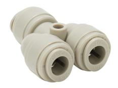
HydroMode potable water push-to-connect fitting, union Y, acetal body, (3) 5/16in tube connection(s), NSF/ANSI 61. Package of 5.
