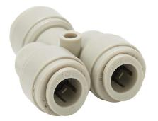
HydroMode potable water push-to-connect fitting, union Y, acetal body, (3) 3/8in tube connection(s), NSF/ANSI 61. Package of 5.
