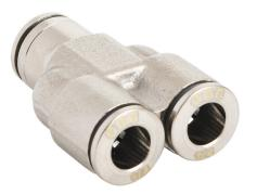
NITRA pneumatic push-to-connect fitting, union Y, nickel-plated brass body, (3) 1/4in push-to-connect connection(s). Package of 5.
