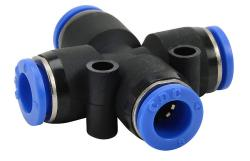
NITRA pneumatic push-to-connect fitting, union cross, thermoplastic (PBT) body, (4) 5/16in (8mm) push-to-connect connection(s). Package of 5.
