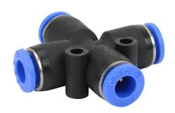
NITRA pneumatic push-to-connect fitting, union cross, thermoplastic (PBT) body, (4) 6mm tube connection(s). Package of 5.
