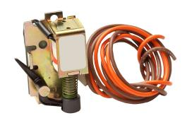
Eaton field installable undervoltage trip, 110-127 VAC sensing range, 18in pigtail. For use with AutomationDirect (Eaton) 600A frame MCCBs.
