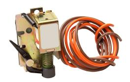
Eaton field installable undervoltage trip, 24 VDC sensing range, 18in pigtail. For use with AutomationDirect (Eaton) 400A frame MCCBs.
