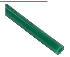
NITRA pneumatic tubing, ether-based polyurethane, dark green, 1/8in outside diameter, 0.062in inside diameter, UV stabilized, 100ft package.
