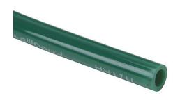
NITRA pneumatic tubing, ether-based polyurethane, dark green, 1/4in outside diameter, 0.156in inside diameter, UV stabilized, 100ft package.
