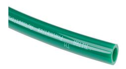
NITRA pneumatic tubing, ether-based polyurethane, dark green, 12mm outside diameter, 5/16in (8mm) inside diameter, UV stabilized, 100ft package.
