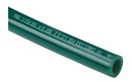
NITRA pneumatic tubing, ether-based polyurethane, dark green, 1/2in outside diameter, 0.328in inside diameter, UV stabilized, 100ft package.
