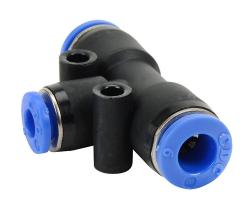
NITRA pneumatic push-to-connect fitting, union tee reducer, thermoplastic (PBT) body, (2) 6mm push-to-connect to (1) 5/32in (4mm) push-to-connect. Package of 5.
