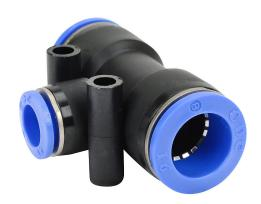
NITRA pneumatic push-to-connect fitting, union tee reducer, thermoplastic (PBT) body, (2) 16mm push-to-connect to (1) 10mm push-to-connect. Package of 3.
