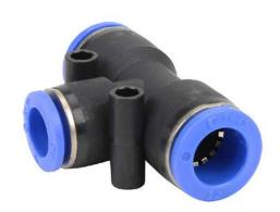
NITRA pneumatic push-to-connect fitting, union tee reducer, thermoplastic (PBT) body, (2) 12mm tube to 10mm tube connection(s). Package of 5.
