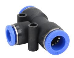
NITRA pneumatic push-to-connect fitting, union tee reducer, thermoplastic (PBT) body, (1) 10mm push-to-connect to (2) 5/16in (8mm) push-to-connect. Package of 5.
