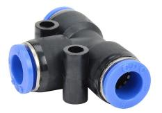
NITRA pneumatic push-to-connect fitting, union tee, thermoplastic (PBT) body, (3) 5/16in (8mm) tube connection(s). Package of 5.
