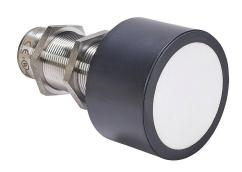
Micro Detectors ultrasonic proximity sensor, tubular, 30mm diameter x 115mm body, 316L stainless steel housing, PNP, (2) N.O./N.C. selectable outputs, 600-8000mm sensing distance, 1 Hz switching frequency, IP67, 5-pin M12 quick-disconnect.
