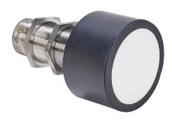
Micro Detectors ultrasonic proximity sensor, tubular, 30mm diameter x 115mm body, 316L stainless steel housing, PNP, 0-10 VDC analog output, N.O./N.C. selectable output, 600-8000mm sensing distance, 1 Hz switching frequency, IP67, 5-pin M12 quick-disconnect.
