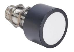
Micro Detectors ultrasonic proximity sensor, tubular, 30mm diameter x 115mm body, 316L stainless steel housing, PNP, 4-20 mA analog output, N.O./N.C. selectable output, 600-8000mm sensing distance, 1 Hz switching frequency, IP67, 5-pin M12 quick-disconnect.
