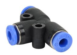
NITRA pneumatic push-to-connect fitting, union tee, thermoplastic (PBT) body, (3) 5/32in (4mm) push-to-connect connection(s). Package of 5.
