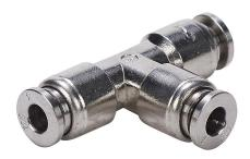
NITRA pneumatic push-to-connect fitting, union tee, 316 stainless steel body, (3) 5/32in (4mm) tube connection(s).
