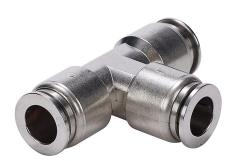
NITRA pneumatic push-to-connect fitting, union tee, 316 stainless steel body, (3) 3/8in push-to-connect connection(s).
