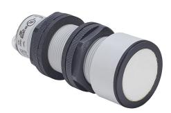
Micro Detectors ultrasonic proximity sensor, tubular, 30mm diameter x 98.8mm body, polybutylene terephthalate housing, PNP, (2) N.O./N.C. selectable outputs, 350-6000mm sensing distance, 1 Hz switching frequency, IP67, 5-pin M12 quick-disconnect.
