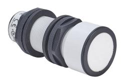
Micro Detectors ultrasonic proximity sensor, tubular, 30mm diameter x 98.8mm body, polybutylene terephthalate housing, PNP, 0-10 VDC analog output, N.O./N.C. selectable output, 350-6000mm sensing distance, 1 Hz switching frequency, IP67, 5-pin M12 quick-disconnect.
