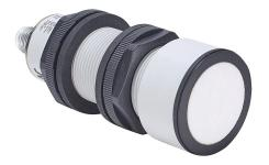
Micro Detectors ultrasonic proximity sensor, tubular, 30mm diameter x 98.8mm body, polybutylene terephthalate housing, PNP, 4-20 mA analog output, N.O./N.C. selectable output, 350-6000mm sensing distance, 1 Hz switching frequency, IP67, 5-pin M12 quick-disconnect.
