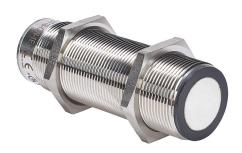
Micro Detectors ultrasonic proximity sensor, tubular, 30mm diameter x 98.8mm body, 316L stainless steel housing, PNP, (2) N.O./N.C. selectable outputs, 250-3500mm sensing distance, 1 Hz switching frequency, IP67, 5-pin M12 quick-disconnect.
