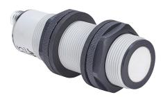
Micro Detectors ultrasonic proximity sensor, tubular, 30mm diameter x 98.8mm body, polybutylene terephthalate housing, PNP, (2) N.O./N.C. selectable outputs, 250-3500mm sensing distance, 1 Hz switching frequency, IP67, 5-pin M12 quick-disconnect.
