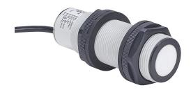
Micro Detectors ultrasonic proximity sensor, tubular, 30mm diameter x 88.8mm body, polybutylene terephthalate housing, PNP, (2) N.O./N.C. selectable outputs, 250-3500mm sensing distance, 1 Hz switching frequency, IP67, pigtail.
