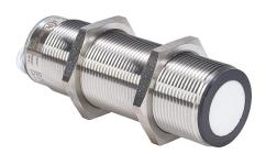
Micro Detectors ultrasonic proximity sensor, tubular, 30mm diameter x 98.8mm body, 316L stainless steel housing, PNP, 0-10 VDC analog output, N.O./N.C. selectable output, 250-3500mm sensing distance, 1 Hz switching frequency, IP67, 5-pin M12 quick-disconnect.
