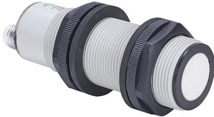
Micro Detectors ultrasonic proximity sensor, tubular, 30mm diameter x 98.8mm body, polybutylene terephthalate housing, PNP, 0-10 VDC analog output, N.O./N.C. selectable output, 250-3500mm sensing distance, 1 Hz switching frequency, IP67, 5-pin M12 quick-disconnect.
