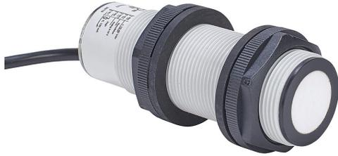
Micro Detectors ultrasonic proximity sensor, tubular, 30mm diameter x 88.8mm body, polybutylene terephthalate housing, PNP, 0-10 VDC analog output, N.O./N.C. selectable output, 250-3500mm sensing distance, 1 Hz switching frequency, IP67, pigtail.
