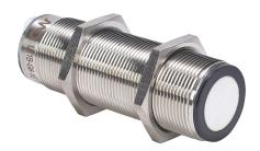
Micro Detectors ultrasonic proximity sensor, tubular, 30mm diameter x 98.8mm body, 316L stainless steel housing, PNP, 4-20 mA analog output, N.O./N.C. selectable output, 250-3500mm sensing distance, 1 Hz switching frequency, IP67, 5-pin M12 quick-disconnect.
