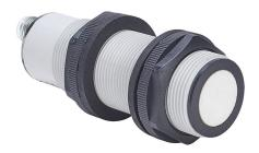
Micro Detectors ultrasonic proximity sensor, tubular, 30mm diameter x 98.8mm body, polybutylene terephthalate housing, PNP, 4-20 mA analog output, N.O./N.C. selectable output, 250-3500mm sensing distance, 1 Hz switching frequency, IP67, 5-pin M12 quick-disconnect.
