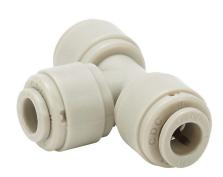
HydroMode potable water push-to-connect fitting, union tee, acetal body, (3) 1/4in tube connection(s), NSF/ANSI 61. Package of 5.
