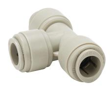
HydroMode potable water push-to-connect fitting, union tee, acetal body, (3) 1/2in tube connection(s), NSF/ANSI 61. Package of 5.
