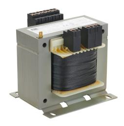
BLOCK control transformer, open core, 800 VA, 1-phase, 208-600 VAC selectable, 115/230 VAC secondary, 50/60 Hz, panel mount.
