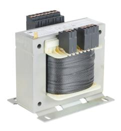
BLOCK control transformer, open core, 500 VA, 1-phase, 208-600 VAC selectable, 115/230 VAC secondary, 50/60 Hz, panel mount.
