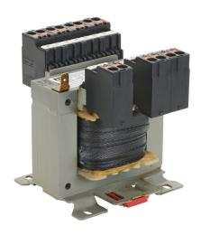
BLOCK control transformer, open core, 40 VA, 1-phase, 208-600 VAC selectable, 12/24 VAC secondary, 50/60 Hz, panel or 35mm DIN rail mount.
