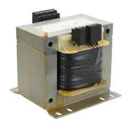
BLOCK control transformer, open core, 2.5 kVA, 1-phase, 208-600 VAC selectable, 115/230 VAC secondary, 50/60 Hz, panel mount.
