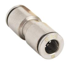
NITRA pneumatic push-to-connect fitting, union straight, nickel-plated brass body, (1) 6mm push-to-connect to (1) 6mm push-to-connect. Package of 5.
