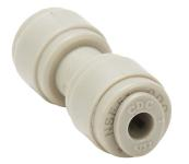
HydroMode potable water push-to-connect fitting, union straight, acetal body, (2) 5/32in tube connection(s), NSF/ANSI 61. Package of 5.
