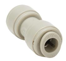
HydroMode potable water push-to-connect fitting, union straight, acetal body, (2) 5/16in tube connection(s), NSF/ANSI 61. Package of 5.
