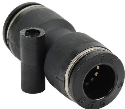
NITRA pneumatic push-to-connect fitting, union straight, thermoplastic (PBT) body, (1) 3/8in push-to-connect to (1) 3/8in push-to-connect. Package of 5.
