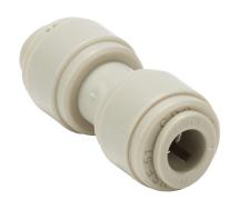
HydroMode potable water push-to-connect fitting, union straight, acetal body, (2) 1/4in tube connection(s), NSF/ANSI 61. Package of 5.
