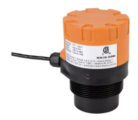
Flowline EchoTouch intrinsically safe reflective ultrasonic liquid level sensor, 9.8ft/3m sensing range, 4-20 mA, 14-28 VDC operating voltage, 2in male NPT process connection.
