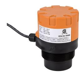
Flowline EchoTouch intrinsically safe reflective ultrasonic liquid level sensor, 4.9ft/1.5m sensing range, 4-20 mA, 14-28 VDC operating voltage, 2in male NPT process connection.
