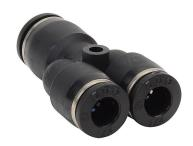
NITRA pneumatic push-to-connect fitting, union Y reducer, thermoplastic (PBT) body, (1) 5/16in (8mm) push-to-connect to (2) 1/4in push-to-connect. Package of 5.
