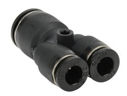
NITRA pneumatic push-to-connect fitting, union Y reducer, thermoplastic (PBT) body, (1) 3/8in push-to-connect to (2) 1/4in push-to-connect. Package of 5.
